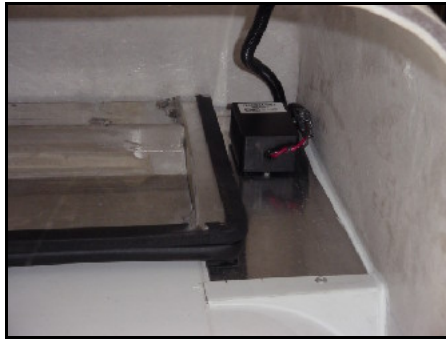
Exterior mounted Temperature sensor (located on the front of the body, beside the damper door)
