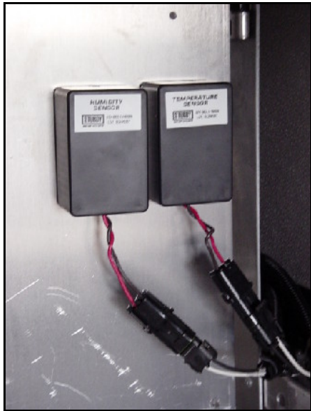
Interior mounted sensors are located on the access doors on the passenger side of the vehicle.
